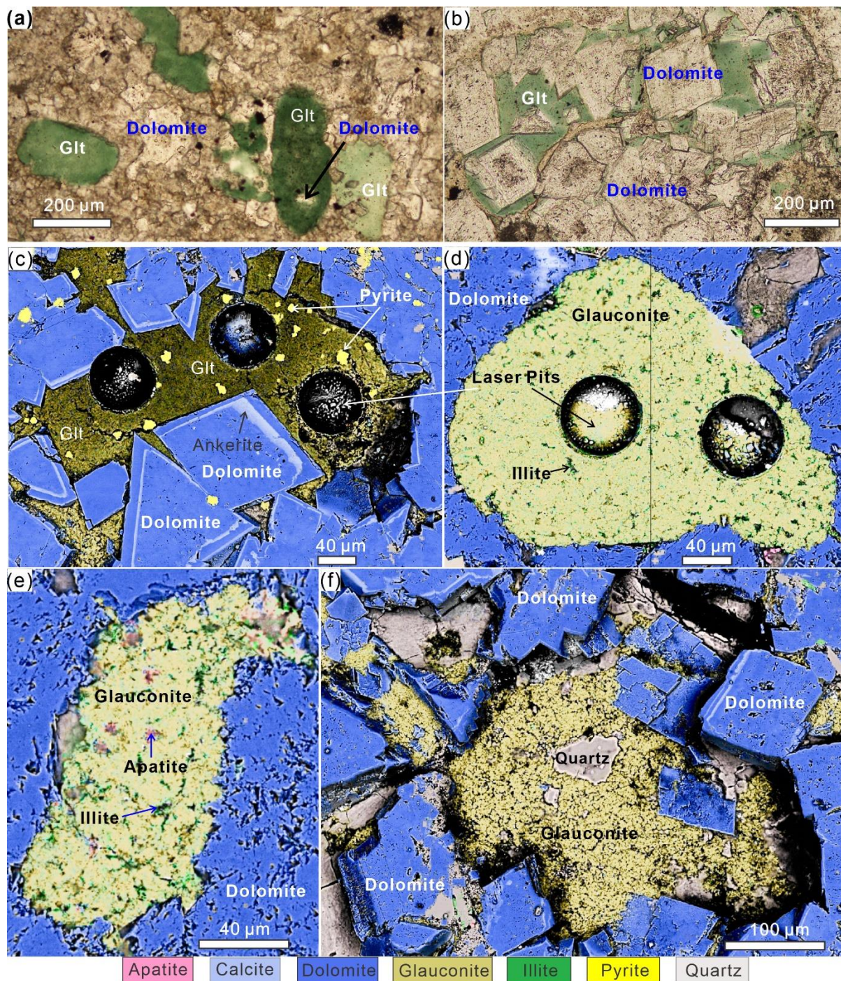
Figure 2. Petrography of glauconite-bearing dolostone samples from the Georgina Basin, Australia: (a)–(b) Transmitted light petrographic images; (c)–(f) Backscattered electron (BSE) images overlaid with mineral mapping from SEM-EDS analysis: (a) Glauconite pellets and/or infill hosted within fine- to medium-crystalline dolostone, showing dolomite micro-inclusions in glauconite (NT2516, Wonarah Formation); (b) Glauconite embedded in a coarse recrystallized dolomite matrix, displaying irregular shapes influenced by adjacent dolomite
