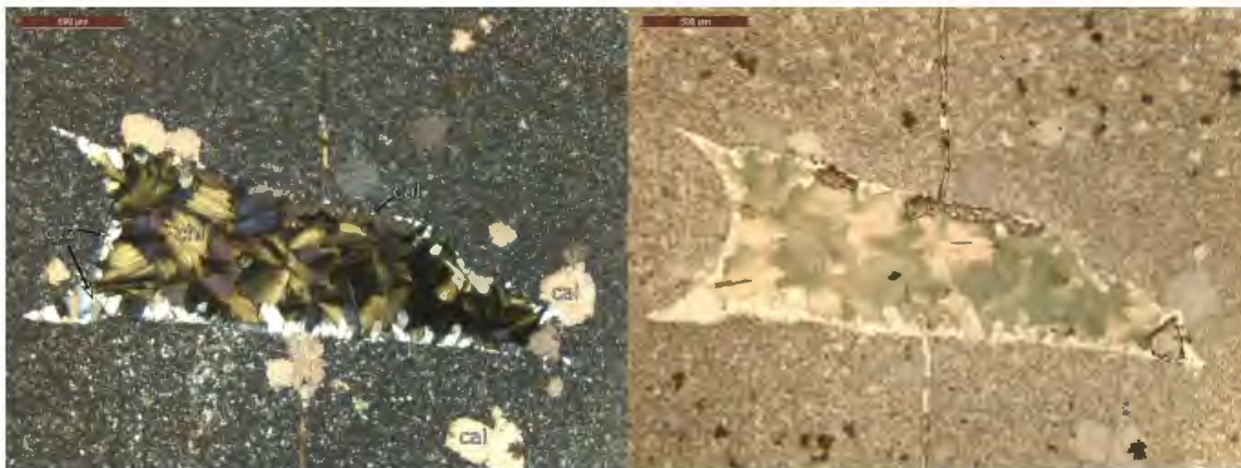
Figure C.8: Crossed-polars (left) and plane-polarised light (right) images of thin section VP003 showing a phenocryst within the enclave entirely replaced by chlorite, rimmed by calcite and quartz.
