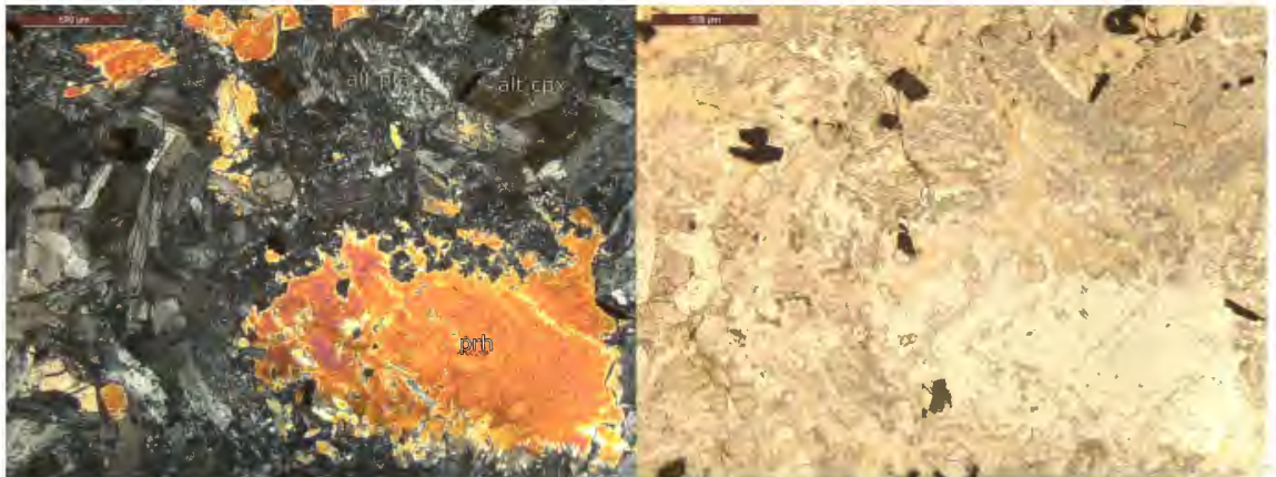
Figure C.22: Crossed-polars (left) and plane-polarised light (right) images of thin section VP009 showing coarse-grained secondary prehnite, altered plagioclase and altered clinopyroxene.
