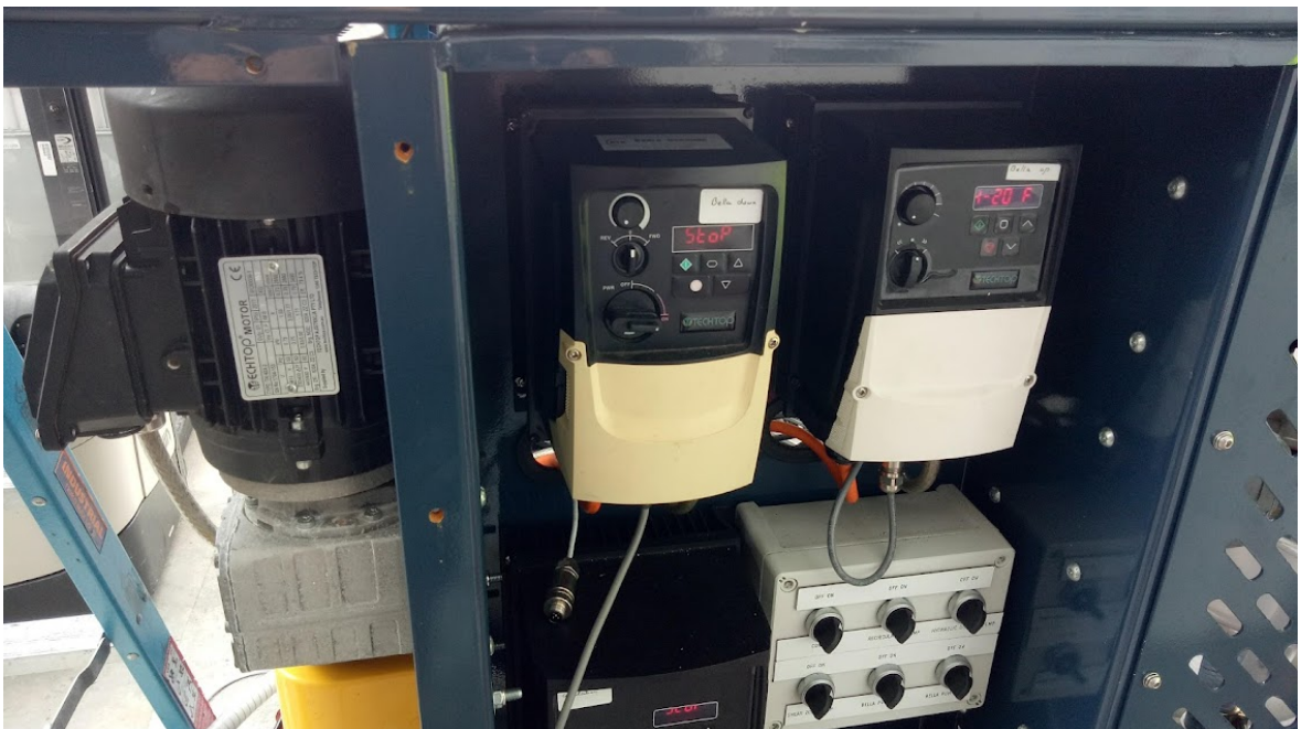
Figure 3.6: VFD and motor used in experiment
