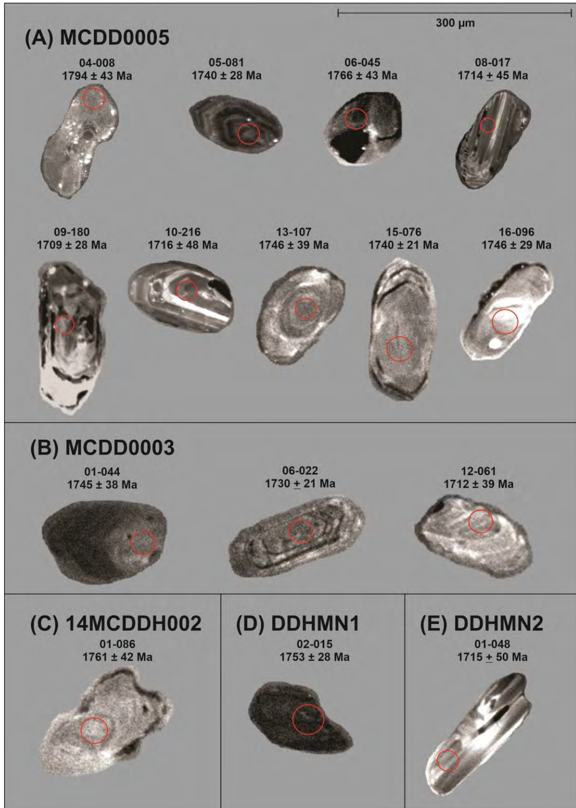
Figure 3: Cathodoluminescence (CL) images of the youngest, near-concordant, detrital zircon grain from the McArthur and Tawallah Groups with their analysis number and ^{207}\text{Pb}/^{206}\text{Pb} age values. Samples are from drill core (A.) MCDD0005, (B.) MCDD0003, (C.) 14MCDDH002, (D.) DDHMN1, and (E.) DDHMN2. U–Pb and REE analyses were taken simultaneously, marked by the red spot in the grains.
