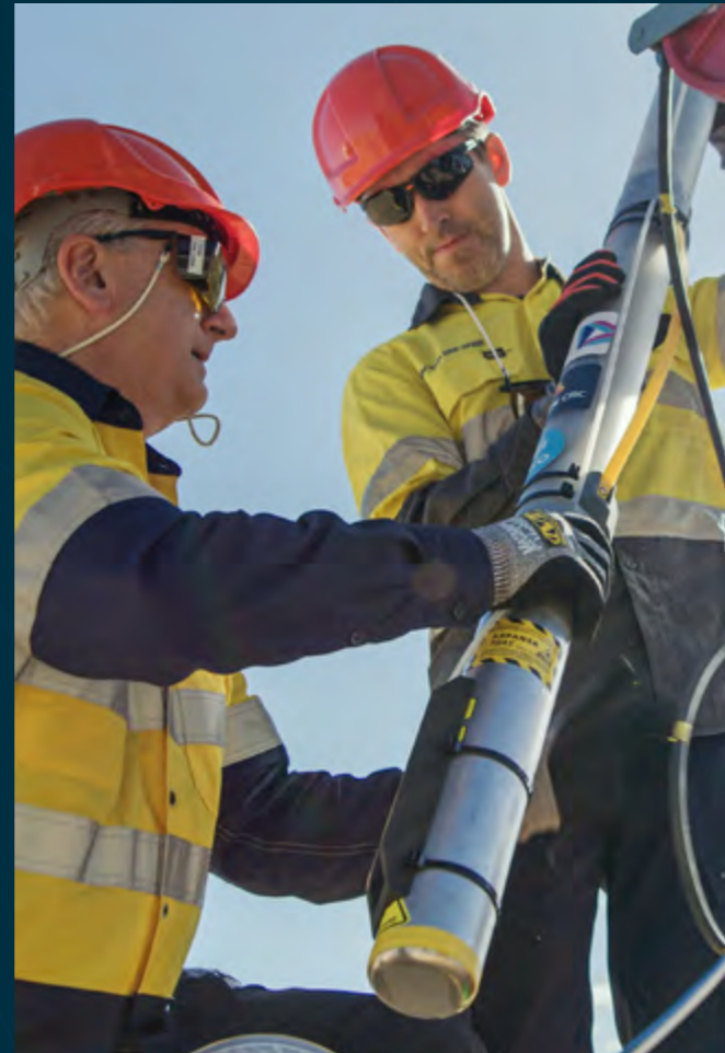
MinEx CRC researchers Steve Tassios, CSIRO (left) and Ben van der Hoek, UniSA (right) during first field trials of the LIBS downhole geochemical tool.
