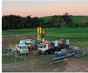
Lakes was to connect and test the multiple linked systems – mechanical, electrical, hydraulic – on the HPS and CT rig in a live drilling scenario and test the platform in complex cover materials.
