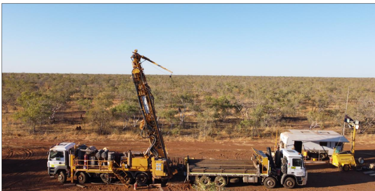
Diamond drill rig on site at the MinEx CRC East Tennant NDI scientific drilling program.
